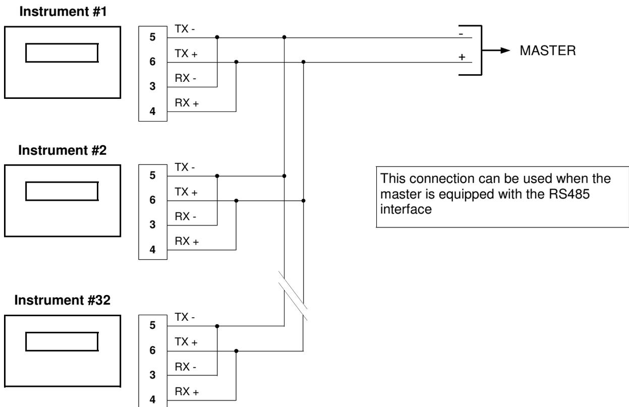
**RS422 or RS485 OUTPUT THROUGH THE SERIAL CONVERTER
