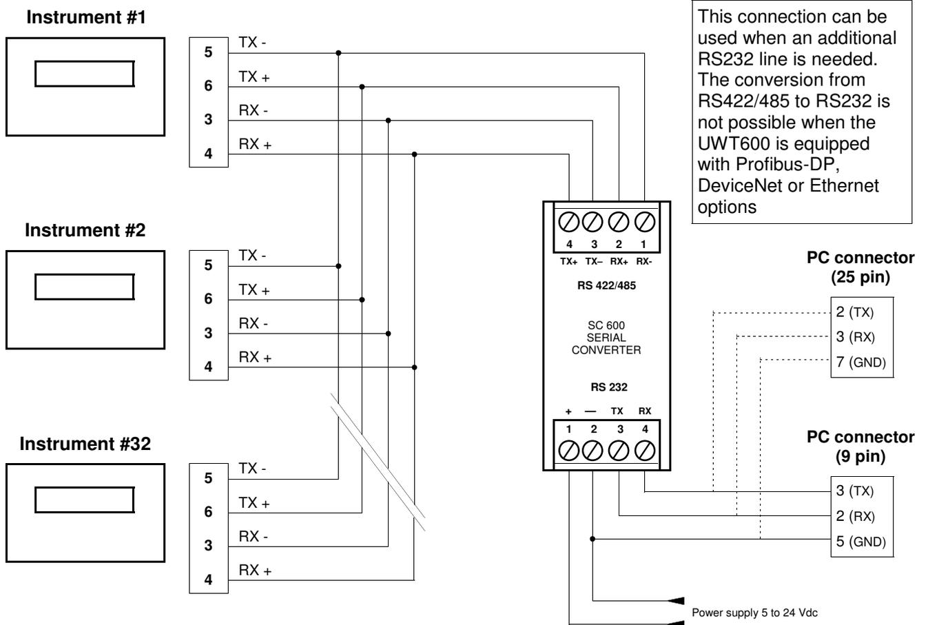
**RS485 CONNECTION TO THE UNI WEIGH H60 REMOTE DISPLAYS - 60 mm. high digits (2.4")**
