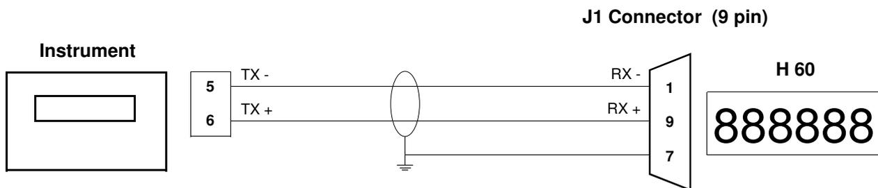
**RS485 CONNECTION TO THE UNI WEIGH H100 REMOTE DISPLAYS 100 mm. high digits (4")**
