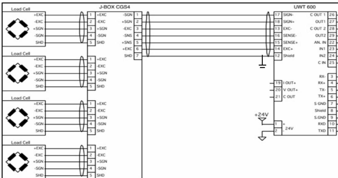
N.B. Connect the load cell shield to terminal 12. Ground the load cell shield on one end only.
