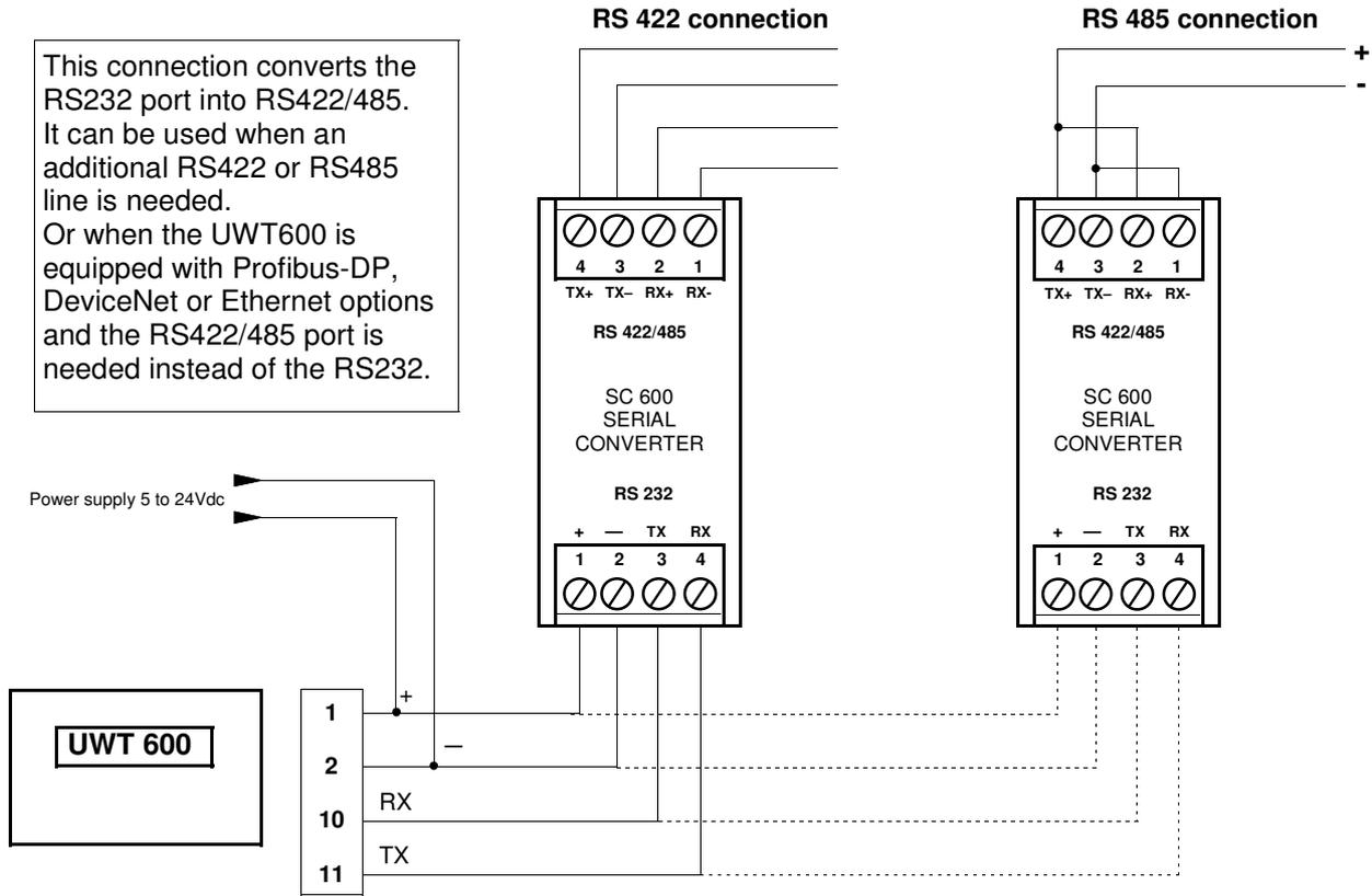
**RS232 OUTPUT THROUGH THE SERIAL CONVERTER (PART NUMBER SC 600 SUPPLIED BY UNI WEIGH)**
